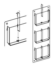
STEP 4. Carefully lift the assembled literature rack up and align the holes on the back panel with the mounted standoffs. Hold the back panel and hand screw all 4 caps into the standoffs.
